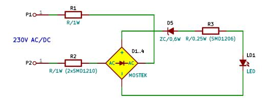
For 24V-AC/DC voltage, power consumption is 0,6 W and for 230V-AC/DC, it is 0,9 W.
